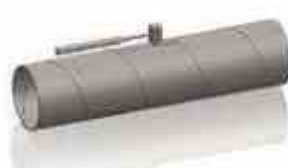
O/S Cross Seam Skelp Welding
