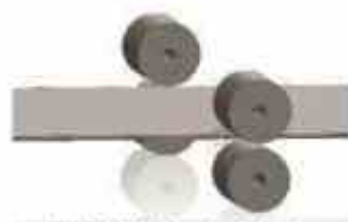
Coil Edge Side Trimming & Cleaning
