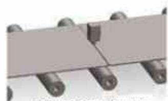
Inside Cross Seam Skelp Welding
